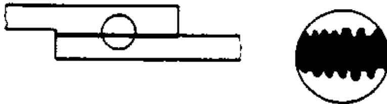
Figure 2/54 Mechanical changes of the adhesive on the workplace surface
