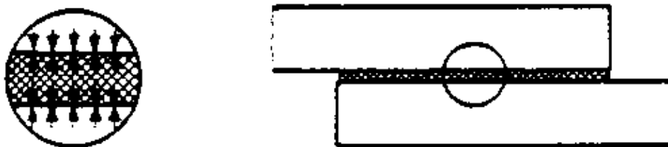
Figure 2/55 Specific adhesion of the adhesive
