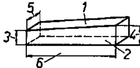
Figure 2/3 Surfaces and dimensions of a key
