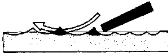
Figure 3/85 Principle of spot scraping
