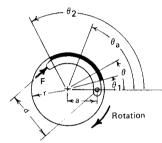
Fig. 8.2.71 Rim brake: internal friction shoe.
