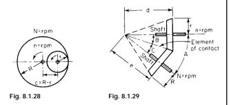
$(N/n + \cos A)$ ; in Fig. 8.1.30,  $\tan B = \sin A/(N/n - \cos A)$ , and  $\tan C = \sin A/(n/N - \cos A)$ . With the above values for the angles *B* and *C*, and the length *d* or *e* of one of the cones, *R* and *r* may be calculated.
