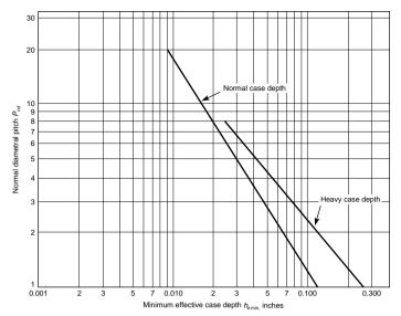
Fig. 8.3.32 Minimum effective case depth for carburized gears  $h_{emin}$ . Effective case depth is defined as depth of case with minimum hardness of 50 RC. Total case depth to core carbon is approximately 1.5 times the effective case depth. (Source: ANSI/AGMA 2001-C95, with permission.)
