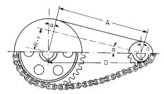
Fig. 8.2.97 Symbols for chain length calculations.
