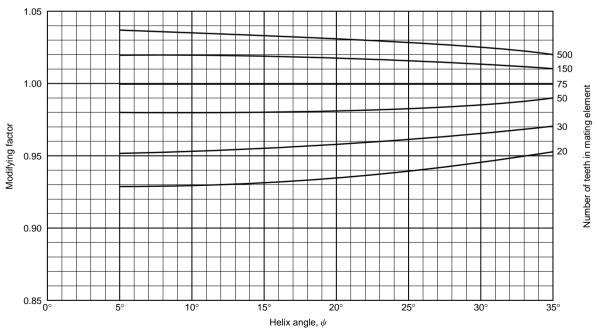
**Fig. 8.3.30** Factor *J* multipliers for 20° normal pressure angle helical gears. The modifying factor can be applied to the *J* factor when other than 75 teeth are used in the mating element. (*Source: ANSI/AGMA 2018-01, with permission.*)
