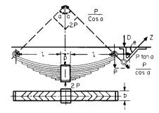
Fig. 8.2.110 Semielliptic springs.
