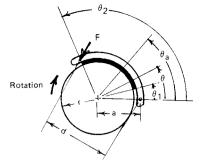
Fig. 8.2.73 Rim brake: external friction shoe.
