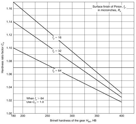
Fig. 8.3.37 Hardness ratio factor C<sub>H</sub> (surface-hardened pinions). (Source: ANSI/AGMA 2001-C95, with permission.)
