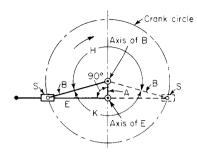
Fig. 8.1.9 Whitworth quick-return motion.
