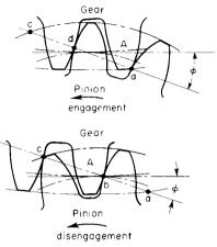
Fig. 8.3.4 Contact conditions at engagement and disengagement.
