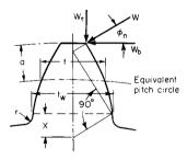
Fig. 8.3.20 Layout for beam strength (Lewis formula).
