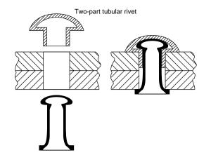
Fig. 8.2.21a Tubular rivets.
