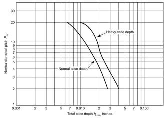
Fig. 8.3.33 Minimum total case depth for nitrided gears  $h_{c \min}$ . (Source: ANSI/AGMA 2001-C95, with permission.)
