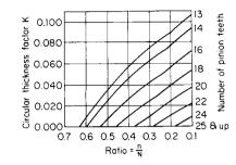
Fig. 8.3.14 Circular thickness factor for straight bevel gears.
