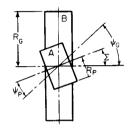
Fig. 8.3.11 Crossed-axis helical gears.
