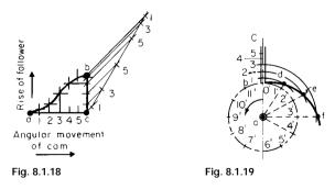
Pitch Line The actual pitch line of a cam varies with the type of motion and with the position of the follower relative to the cam's axis. Most cams as ordinarily constructed are covered by the following four cases.
