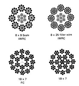
Fig. 8.2.124 Cross section of some rotation-resistant wire ropes. (Reproduced from "Wire Rope User's Manual," AISI, by permission.)
