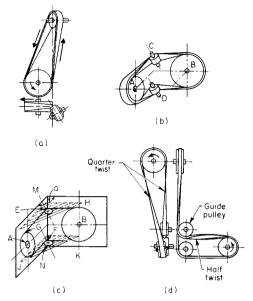
Fig. 8.2.87 Arrangements for flat-belt drives.
