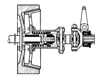
Fig. 8.2.52 Cone clutch.
