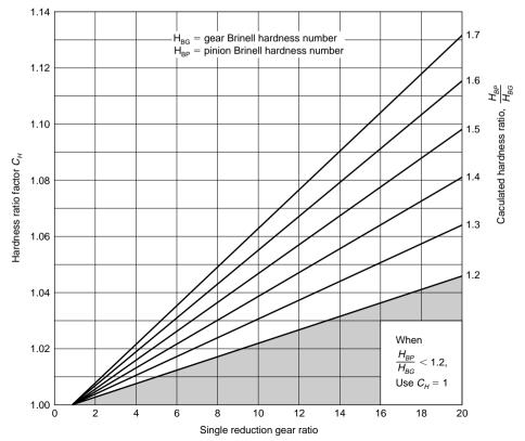
Fig. 8.3.36 Hardness ratio factor C<sub>H</sub> (through-hardened). (Source: ANSI/AGMA 2001-C95, with permission.)
