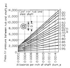
Fig. 8.2.85 Press-fit pressures between cast-iron hub and shaft.
