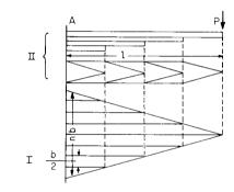
Fig. 8.2.107 Laminated triangular plate spring.
