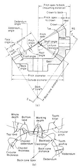
Fig. 8.3.13 Geometry of bevel gear nomenclature. (a) Section through axes; (b) view along axis Z/Z.
