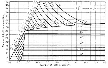
Fig. 8.3.5 Contact ratio, spur gear pairs-full depth, standard generated teeth, 141/2° pressure angle.
