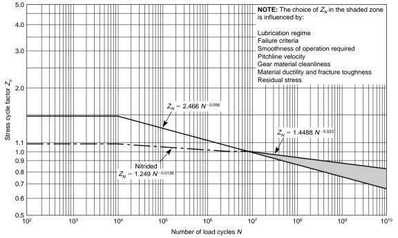
Fig. 8.3.35 Pitting resistance stress cycle factor Z<sub>N</sub>. (Source: ANSI/AGMA 2001-C95, with permission.)
