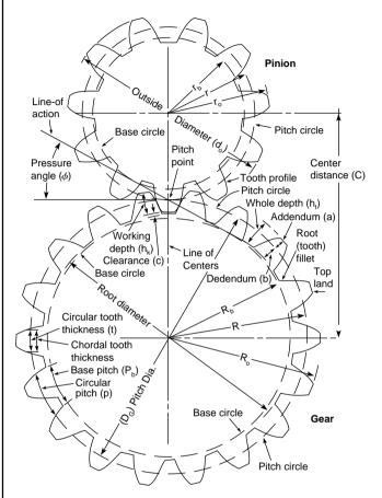
Fig. 8.3.1a Basic gear geometry and nomenclature.
