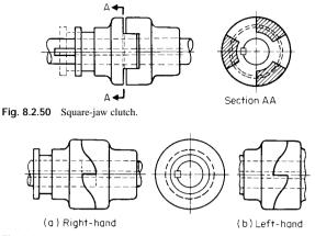
Fig. 8.2.51 Spiral-jaw clutch.
