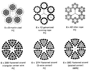
Fig. 8.2.125 Some special constructions. (Reproduced from "Wire Rope User's Manual," AISI, by permission.)
