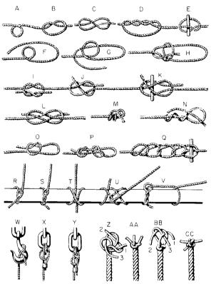
Fig. 8.2.130 Knots, hitches, and bends.
