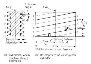
Fig. 8.3.19 Cylindrical worm geometry and design parameters.
