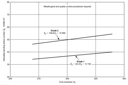
**Fig. 8.3.40** Allowable bending stress numbers *s<sub>at</sub>* for nitrided through-hardened steel gears (i.e., AISI 4140 and 4340). (*Source: ANSI/AGMA 2001-C95, with permission.*)
