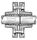
Fig. 8.2.35 Flanged face coupling.
