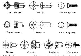
Fig. 8.2.10 Driving recesses. (Adapted, with permission, from Machine Design.)
