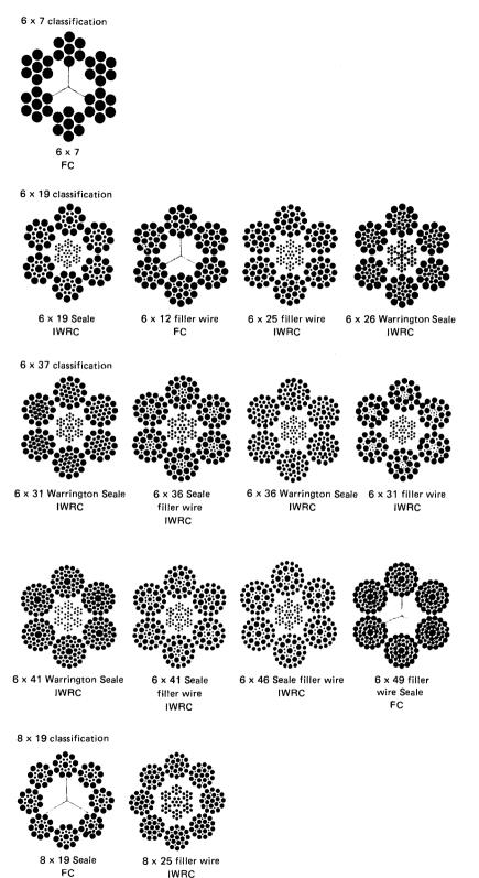
Fig. 8.2.123 Cross sections of some commonly used wire rope construction. (Reproduced from "Wire Rope User's Manual," AISI, by permission.)
