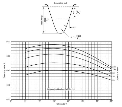
Fig. 8.3.28 Geometry factor J for  $20^{\circ}$  normal pressure angle helical gears. (Standard addendum, full fillet hob.) (Source: ANSI/AGMA 2018-01, with permission.)
