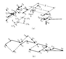
Fig. 8.2.102 (a) Forces and torques; (b) force polygons.
