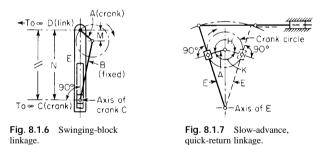
8.1.9) may be found by locating, in the case of the swinging block (Fig. 8.1.7), the two tangent points (t) and measuring the angles H and K made by the two positions of the crank A. If H and K are known, the axis of E may be located by laying off the angles H and K on the crank circle
