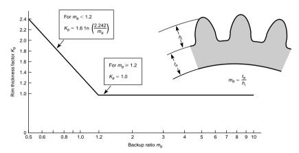
Fig. 8.3.38 Rim thickness factor K<sub>B</sub>. (Source: ANSI/AGMA 2001-C95, with permission.)
