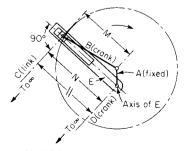
Fig. 8.1.8 Turning-block linkage.
