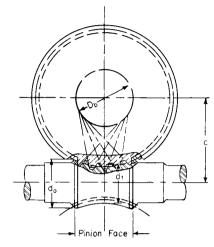
Fig. 8.3.18 Double enveloping worm gearing.
