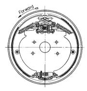
Fig. 8.2.72 Internal brake.
