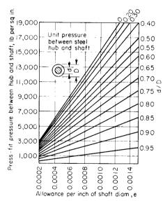
Fig. 8.2.83 Press-fit pressures between steel hub and shaft.
