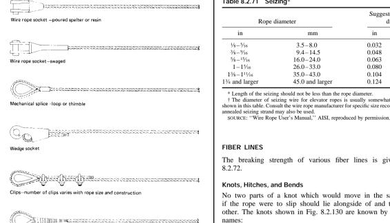
Fig. 8.2.129 End fittings, or terminations, showing the six most commonly used. (Reproduced from 'Wire Rope User's Manual," AISI, by permission.)
