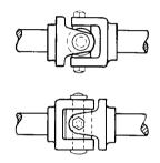
Fig. 8.2.45 Hooke's universal joint.
