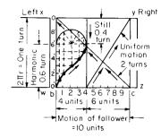
Fig. 8.1.22 Cylindrical cam.
