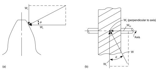
Fig. 8.3.21 Forces on spur and helical teeth. (a) Spur gear; (b) helical gear.
